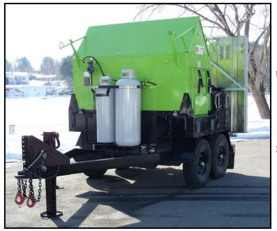
The infrared heating chamber is lowered over the asphalt surface and uses infrared light rays to heat the asphalt. Once heated, the asphalt can be raked around and luted.
