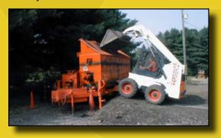
A Feed auger moves RAP millings across the hopper for delivery to the pugmill below. The auger speed is easily adjusted from the control panel. A faster feed rate is set when producing cold patch, while a slower feed rate is typically used when recycling.
