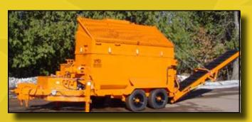
Millings are loaded into the 10 foot wide preheated hopper (charging bin) using a bucket loader. The steel screen prevents oversize pieces from entering the top load bin while acceptable size material passes directly into the load bin.
