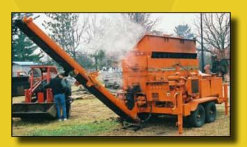
Hot mix discharges from the rear of the recycler via the conveyor. The 14' high off-load conveyor can reach a height of 126" making it easy to load your larger triaxle dump trucks with recycled hot mix or cold patch.
