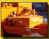
The mixing chamber is heated by 4 diesel fired burners, providing indirect heat via heat conduction through the mixing chamber walls. This prevents the flames from contacting the millings, reducing smoke emissions and maximizing the retention of essential tar oils.
