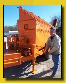
Once the pre-heat hopper is loaded, the burner is set to 'on' and the kettle thermostat adjusted to the desired temperature. The feed auger and pugmill mixer speeds are adjustable and can be set based upon mix design, moisture content and desired output temperature. No further steps are required to operate the recycler.
