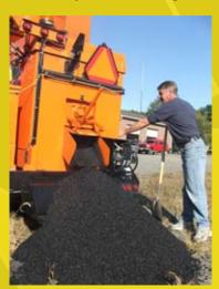
"Hose' position and spray tack to the repair site using the spray wand. Available options include a hose reel, overhead hose boom and an overnight heater.
