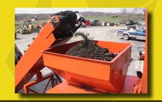
**Recycling**: RAP material enters the recycler from the loading hopper. Here the RAP is mixed, heated and broken down. Moisture is then removed and additive may be mixed in as the RAP is recycled to the target
