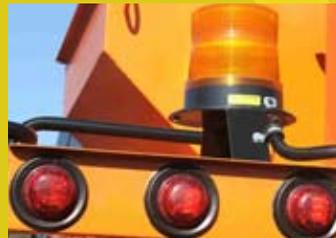
**Lights** are all sealed beam. Options include 2 or 4 lamp LED, strobe light and light bar.
