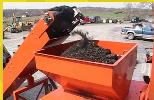
**Recycling:** RAP material enters the recycler from the loading hopper. Here the RAP is mixed, heated and broken down. Moisture is then removed and additive may be mixed in as the RAP is recycled to the target temperature. The PT 10-120 produces 1/2 ton batches
