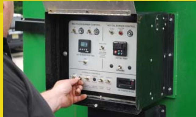
"Hose" position and spray tack to the repair site using the spray wand. Available options include a hose reel, overhead hose boom and an overnight heater.
