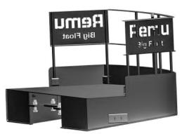
REMU counterweight can be equipped with an inbuilt fuel tank to refuel the original.
