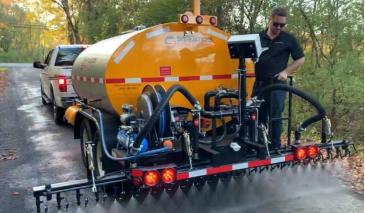
Truck & Trailer - computer monitor, remote on/off, radar guided application rate
