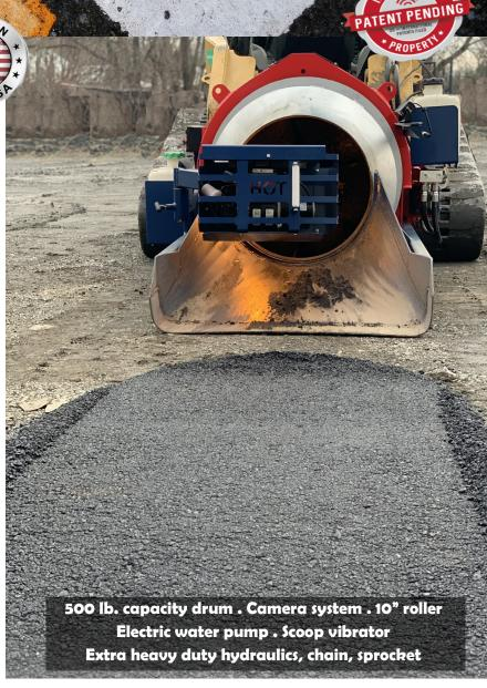
Portable asphalt recycler. Skidsteer attachment. 400Lbs in 15 minutes
